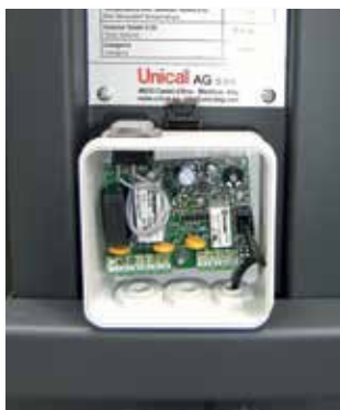
■ Temperature regulation system, with NTC sensor
