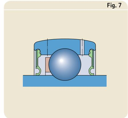
SKF E2 Y-bearings are supplied filled with a special low-noise, low-friction SKF grease (→ [table 3](#)).
