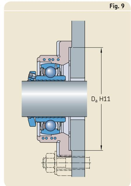
Recommended fastener metric thread sizes are listed in product tables. SKF E2 Y-bearing units with plummer block housings have two bolt holes in their base for attachment bolts. SKF E2 Y-bearing units with a flanged housing have a recess (→ **fig. 9**), at the back for accurate positioning, on an appropriate centring ring provided by one of the following methods:
